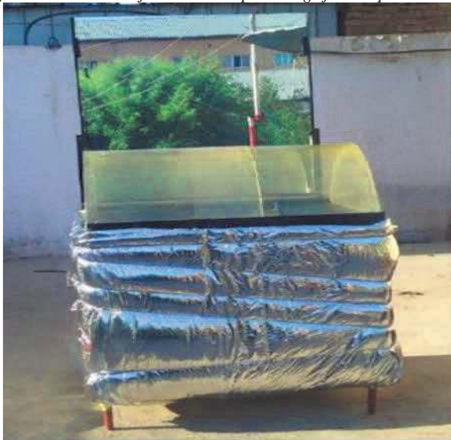
Fig.10. Experimental solar installation for the thermal processing of municipal solid waste.
